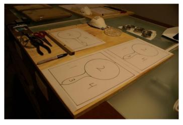
**Pattern number 1** is used to cut its individual pieces, with special lead pattern sheers (these have a well in one of the blades to capture the black line of the pattern accommodating for the lead). These pieces are used as templates for glass cutting.
